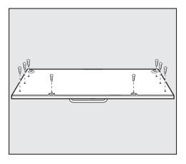
To Screw the removed panel to the custom panel with the eight screws.
